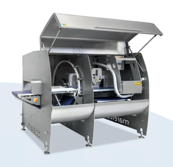
A PORTIO 3 adds two lateral cameras to the PORTIO 1. This allows the machine to improve the scanning and cover blind spots at the side of the product that cannot be detected by the top camera only. It is used for accurately portioning red meat, whole fish or any product with an irregular shape, in a vertical way. The machine can be equipped with the options mentioned on page 20.
