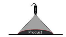
The PORTIO 3 uses the same top camera in combination with two cameras from the side. This allows for scanning the contours of more rounded products, to prevent blind spots on the edges. Typical products are meat, sausages or whole fish.
