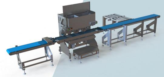
Each salmon is measured by a high quantity of lasers to determine its physical size and direction on the belt. A proportionate amount of salt is applied specific to each fillet's location (belly side left or right). The machine can also double as a spice doser and combine salt and spice as in production of gravadlax.
