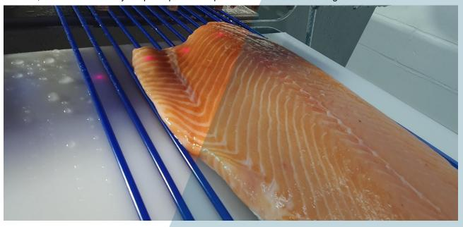
Each salmon is measured with a series of lasers to determine its physical size and a proportionate amount of salt is applied. As this is kept in line the moving of fillets onto rakes after drysalting is the only manual step needed. Next step in the process is curing.
